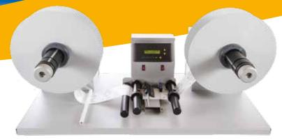
The control panel incorporates a 2-line, 20 character display and 7 function keys for programming:
