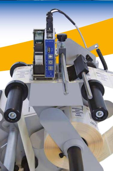
DWR ROUND can also be equipped with an inkjet marker with HP technology for printing variable data such as date and time, barcodes and text with a maximum height of 12.7 mm, a resolution of 300 dpi and speed synchronised with the label supply speed. The text, prepared on a PC using the supplied software, is transferred to the marker via a USB stick.
